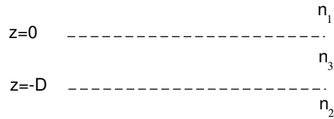
Fig. 3. Three layer geometry with polarization source in medium with index n_3 .
